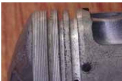
**Abb. 1-16:** Kolbenringnuten
